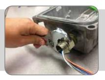
Thread the front piece of the node entry connector into the node housing. Use the crescent wrench to ensure that it is tight and makes a good seal. Use caution not to over tighten and damage the threads on the node housing.
