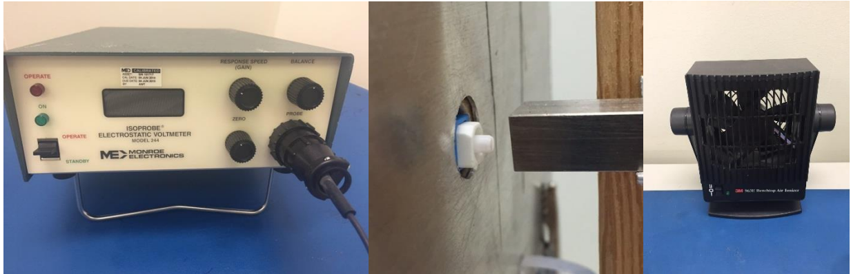
Photos of the core equipment used in static testing
